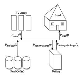
Figure: nGrid architecture with battery, fuel cell, solar, and load
